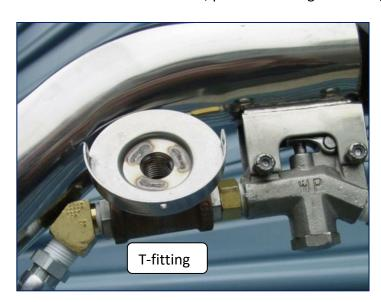
Next, remove the trigger valve and screw it into the back of the T-fitting Line the whole assembly up with the back screw of the hanger to check the fit.
